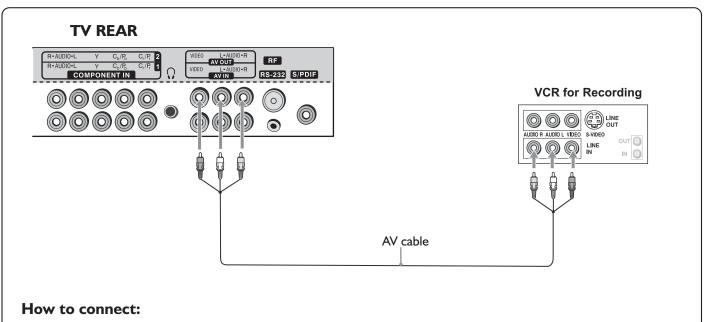
Connect the Audio/Video cables between the Audio (L/R)/Video jacks on the unit and VCR.
